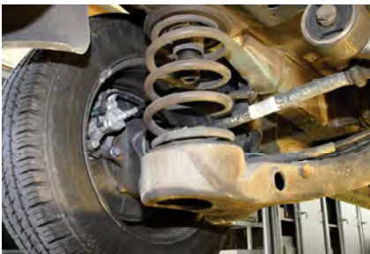
Figure 2.5 Vehicle suspensions can act like mass–spring systems.
