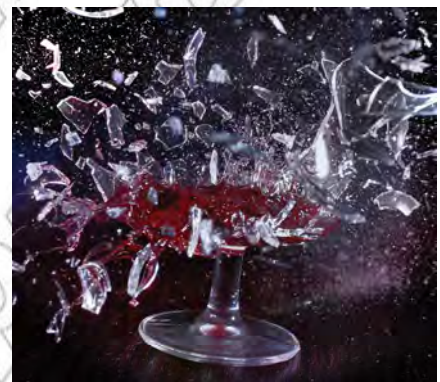
Figure 2.24 Glasses can be made to shatter if they vibrate at their resonant frequency
